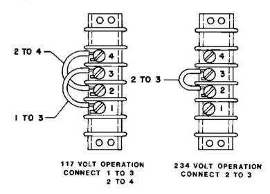
When the AL-80 is operated on 117 volts A.C. be sure the wiring between the fuse box and the A.C. outlet is of adequate gauge to provide the current required without a significant drop in line voltage. No. 12 wire is recommended.
