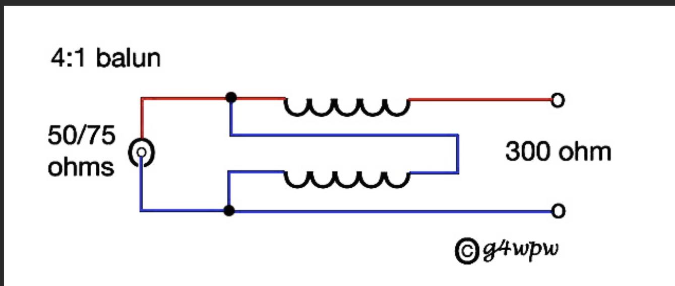
The construction for this balun uses the same principles as the previous one use a 300 ohm carbon resistor to check the swr, this should again be 1:5 - 1 or less.
