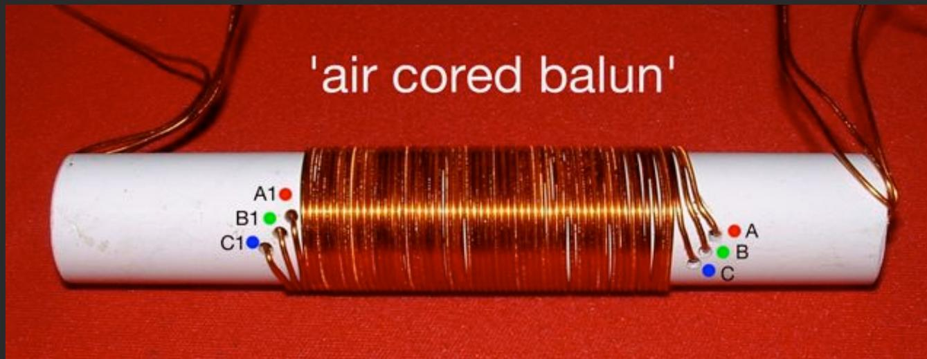
The finished balun's should be encased or insulated from the elements.
