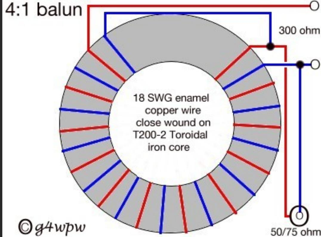
a small gap must be left between the start and finish of the windings
