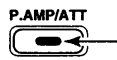
Lights green while the preamp is activated; lights red while the attenuator is activated.
