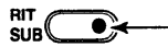
Lights red while the RIT function is activated; green while the SUB DIAL function is activated.
