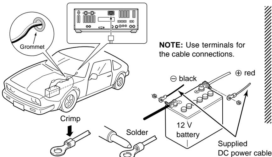
**⚠ WARNING NEVER connect** to a battery without supplied DC fuses, otherwise a fire hazard may occur.
