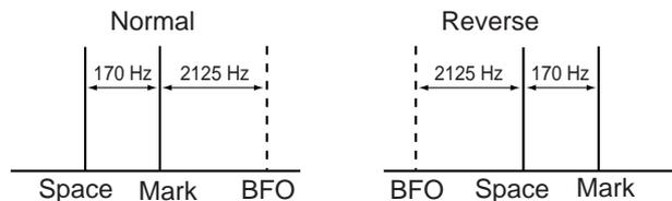
◇ RTTY filter/Twin peak filter
