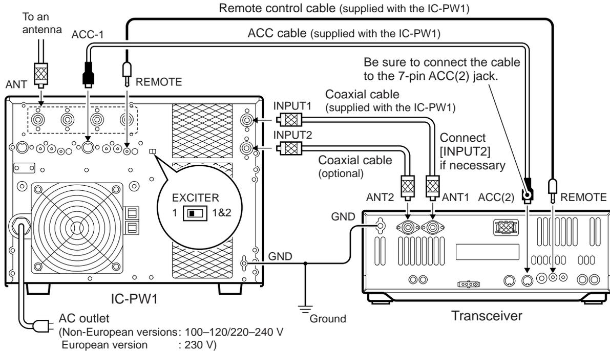
Turn OFF the transceiver's antenna tuner while tuning the IC-PW1's tuner.
