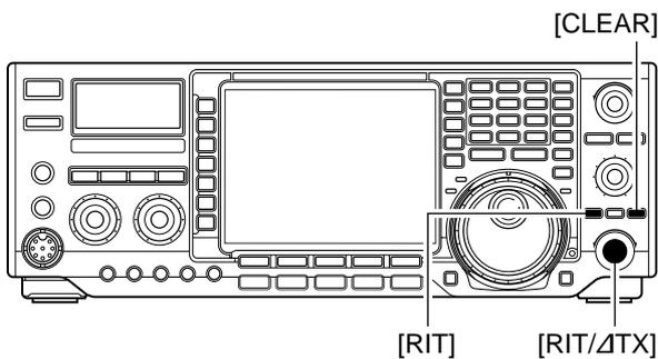
When RIT and  $\Delta$ TX are ON at the same time, the [RIT/ $\Delta$ TX] control shifts both the transmit and receive frequencies from the displayed frequency at the same time.
