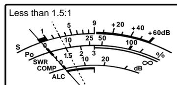
▨ The built-in antenna tuner matches the transmitter to the antenna when the SWR is lower than 3 : 1.
