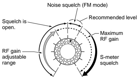
**•When functioning as RF gain control**
