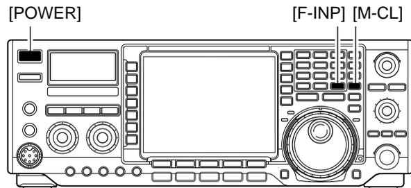
Under cooler temperatures, the LCD may appear dark and unstable after turning power ON. This is normal and does not indicate any equipment malfunction.
