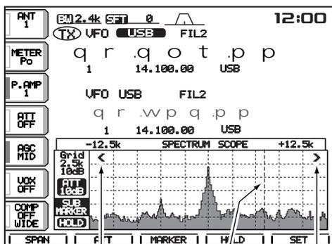
Appears when the marker is out of range.      Sub readout or TX marker      Appears when the marker is out of range.
