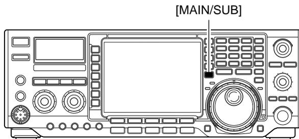
➔ Push [MAIN/SUB] to select access to the main or sub readout.
