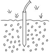
Use the heaviest gauge wire or strap available and make the connection as short as possible.
