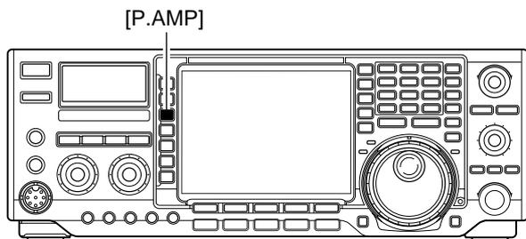
➔ Push [P.AMP] several times to set the preamp OFF, preamp 1 ON or preamp2 ON.
