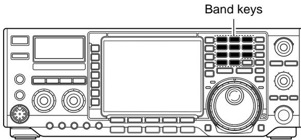
The triple band stacking register provides 3 memories in one band. 3 sets of a frequency and operating mode on each band are automatically stored when used.
