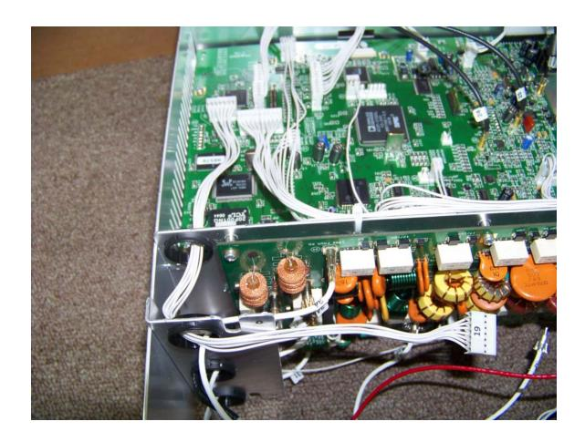
9. Pull the #19 cable out from the grommet that was holding it in place as shown in step 8. Unfurl the cable to its full length, then thread the connector end through the two plastic grommets as shown above. Leave this cable unplugged. It will be plugged into the autotuner board in a later step.
