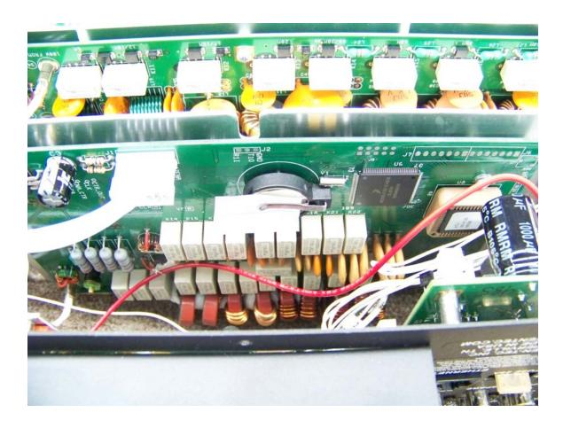
13. There is a small piece of paper inserted between the battery clip and the battery used in the autotuner. Remove this piece of paper. The autotuner installation is now complete.
