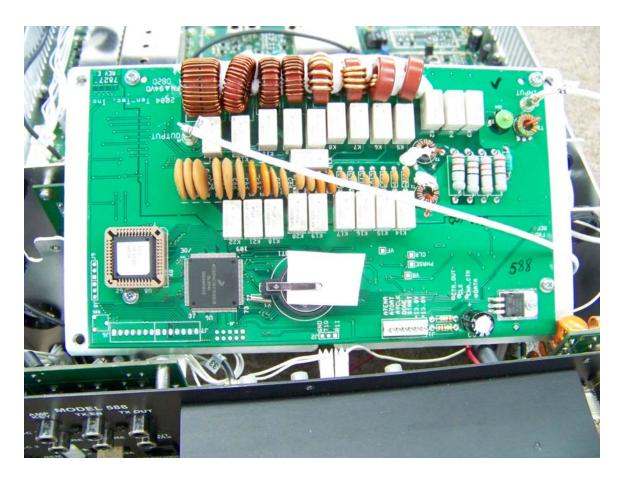
10. With the radio returned to right side up, retrieve the tuner board and shield assembly and turn it correct side up as shown. Plug cable #32 into the connector marked OUTPUT. Plug cable #31 into the connector marked INPUT as shown in the illustration. Please note with the board correct side up for installation that the printing on the PC board is oriented in the other direction and will be shown upside down (see photo).
