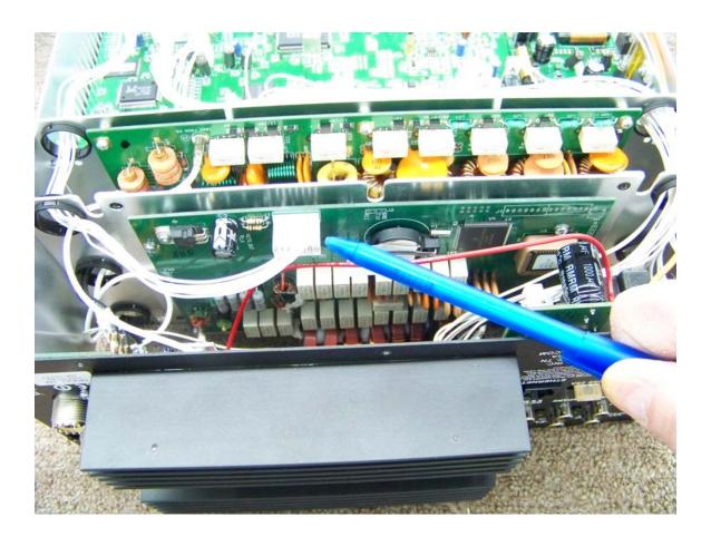
12. Turn transceiver upside down. Install the remaining two black screws that were removed in step 3. The #19 cable that was routed to the back of the radio in step 9 is now ready to be plugged into connector J1. (Pen used as pointer).
