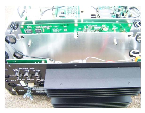
3. This is the rear tuner shield, with standoffs already installed to mount the tuner. There are 4 small black Philips screws holding the plate in place. Remove the first two shown in each corner here, then turn the radio upside down and remove the remaining two. Turn the radio right side up after the bottom two are removed.
