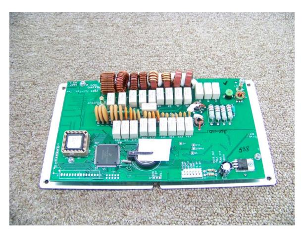
5. Remove the autotuner board from the packing kit and place it onto the tuner shield as shown above. 4 screws, Ten-Tec part #60069 are provided in the packing kit to attach the tuner board to the shield. There is only one possible correct orientation of the board to the shield due to the way the standoffs are set on the board. An incorrect installation will have the circuit board hanging partially off the tuner shield.
