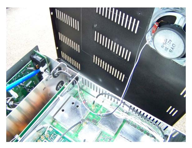
2. Use caution when removing the top cover from the chassis. The internal speaker connection wire can be broken off easily if care is not exercised. The speaker wire is connected to connector 9B just under the external speaker jack as pointed out in the above photo. Pull the socket off the connector and pull the wire out from the black grommets. Set top cover with speaker intact aside.
