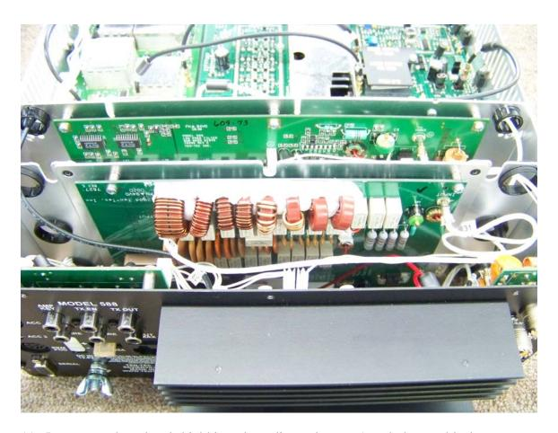
11. Insert tuner board and shield into the radio as shown. Attach the two black screws removed in step 3 into the two corners of the shield.
