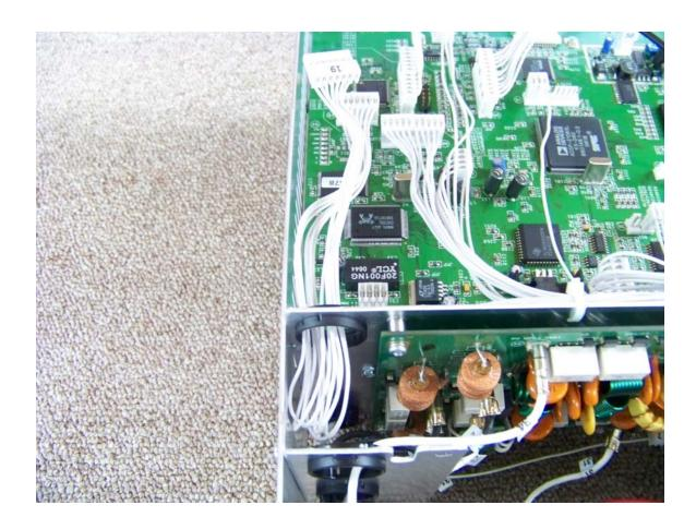
8. Turn the radio upside down. Along the left side of the radio is a multi-wire cable bundle with an unplugged connector marked 19 on one end that is partially tucked inside a plastic grommet.
