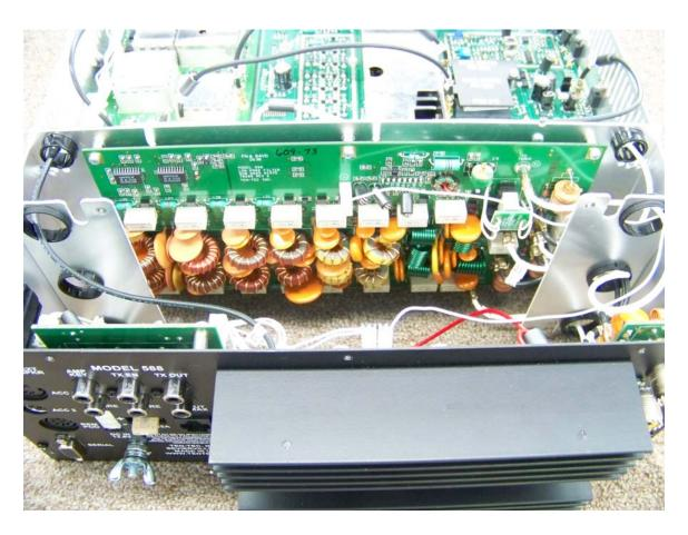
4. This is the view of the rear low pass filter board after the tuner shield has been removed.
