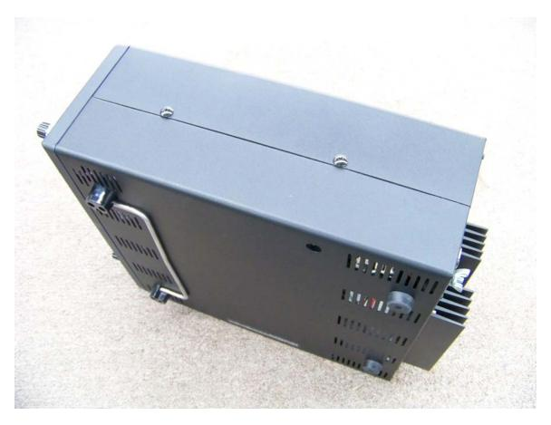
1. Disconnect transceiver power cable from rear. Remove top and bottom cover. There are 2 large black Philips screws on each side of the case. Remove these 4 screws. Around the rear perimeter of the top and bottom covers are #10 Torx screws. Use the provided Torx wrench to remove them.
