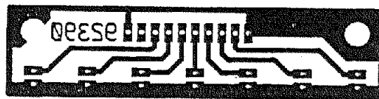
FIGURE 4-29. 81423 BANDSWITCH LED BOARD CIRCUIT TRACE
