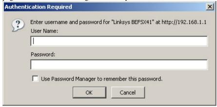
If you do see the prompt for the username / password for the router, or you see the router's configuration setup, then you have the proper IP address.
