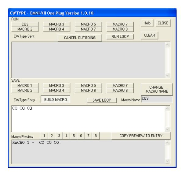
The Macros can be stacked. Meaning that you can click on RUN "MACRO 2", and while it is still running, click on RUN "MACRO 5". Macro 2 and 5 will both run to completion in the order of the data in 2 first, then 5.
