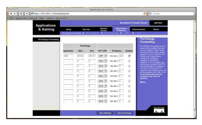
Enter an application name (we chose 588). Then enter a port range. For the OMNI-VII, we use 6 ports, starting with the UDP CMD port. So enter in Start=49152, and End=49157. Make sure the TCP/UDP selection is only on UDP. Set the IP address to the ending number we chose which is .123. Then click on Enabled, and Save Settings.
