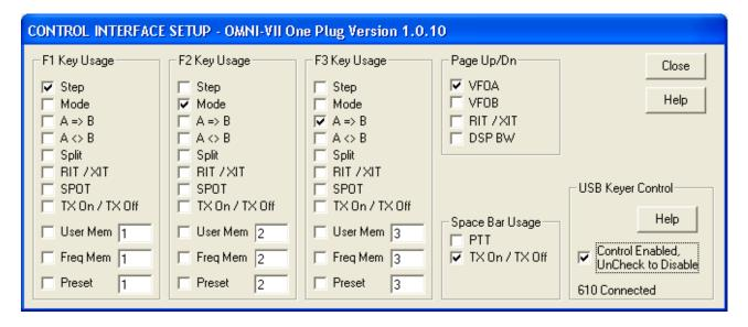
Below shows what the CONTROL IF window will show when the 610 is enabled, yet the 610 has not been annunciated by the PC:
