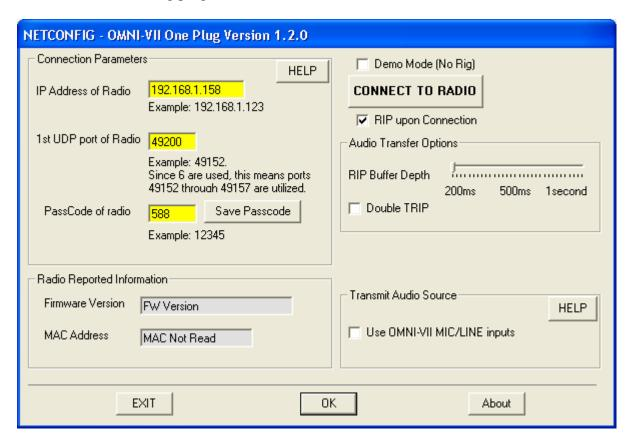
The OMNI-VII One Plug program allows you to run the program and see what controls are available and how they work without actually connecting to a radio. To do this, you can enter "Demo Mode", by left-clicking the mouse on the "Demo Mode" Checkbox, then click OK. You will then be able to see the entire program, but no radio is required.
