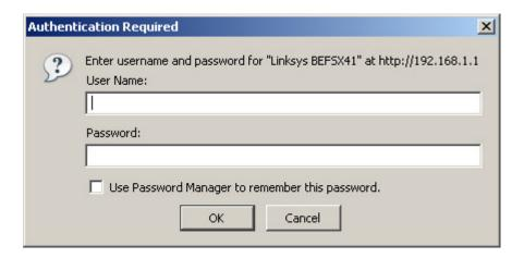
If you do see the prompt for the username / password for the cable modem, or you see the cable modem's configuration setup, then you have the proper IP address.
