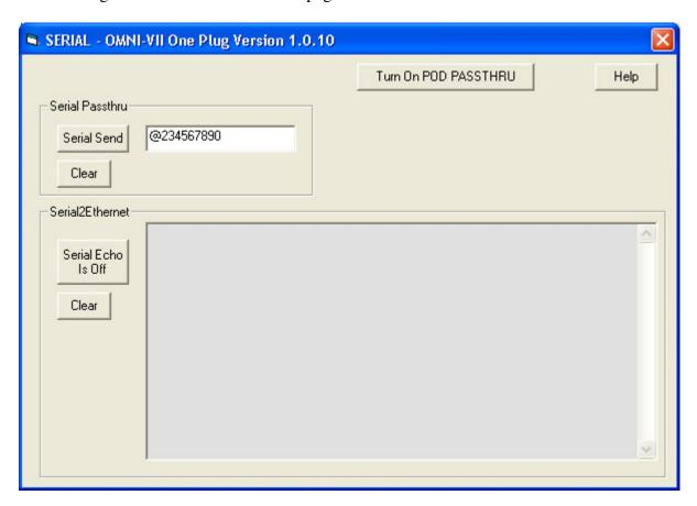
Simply connect up the OMNI\_VII serial port to a computer that is running a terminal emulator such as hyperterm or procomm. Type into the text box next to the SERIAL SEND button a text string you want to go out the serial port, then click on SERIAL SEND, and you will see it arrive at the other computer's hyperterminal program.
