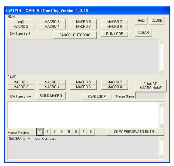
With the CWType Interface, to send CW, left-click the mouse on the CWTPE Entry Window, and then start typing with the local keyboard. The characters are then sent to the radio for it to send out at the selected CW settings.
