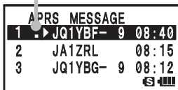
APRS MESSAGE Screen (Display of when ACK is being received)
